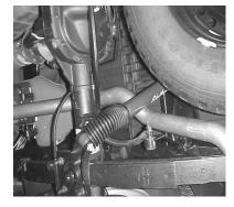
INSERT WELDED HANGER INTO THE RUBBER GROMMET.
